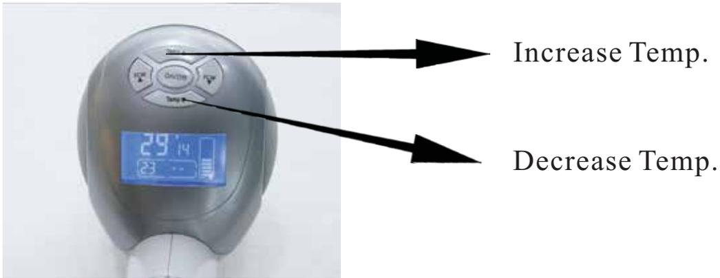
Remark: When the temp display "--", It means Stop cooling ,
